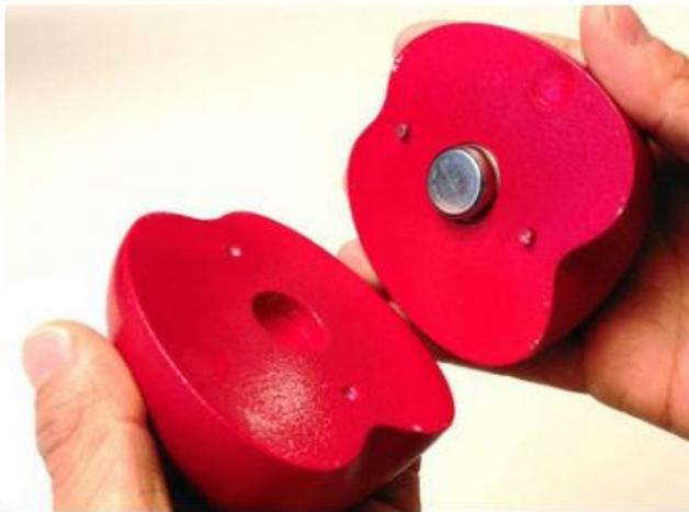
One of Empa's temperature sensors in the shape of a Braeburn apple (Empa)
